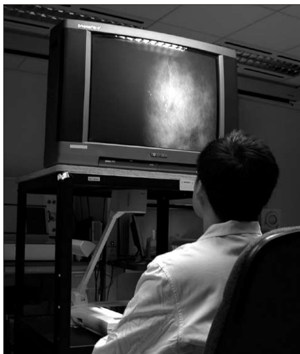
Figure 2. Analogue magnification of microcalcifications achieved by using a video visualiser and a television.
