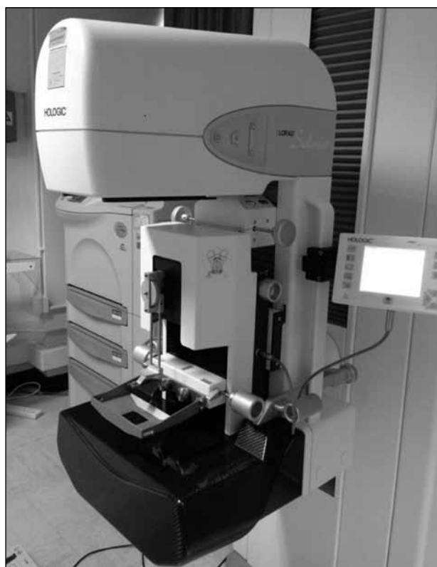
Figure 2. Digital add-on unit (Digital Stereo Loc, Hologic) used in our breast centre.
